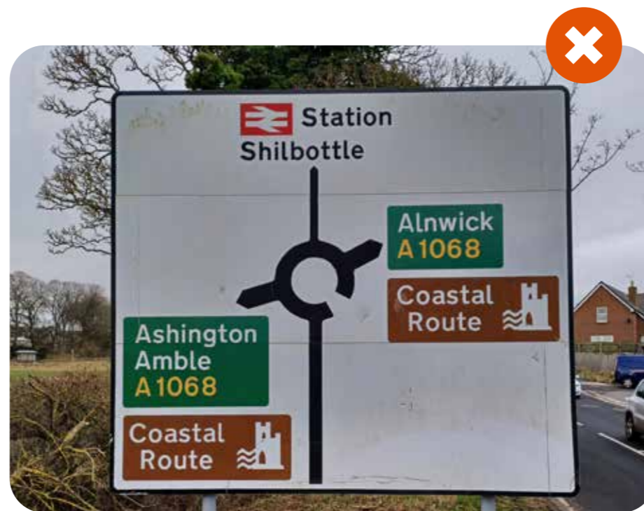
Sign should use the Coastal Route logo only, to allow overall sign size to be reduced.
