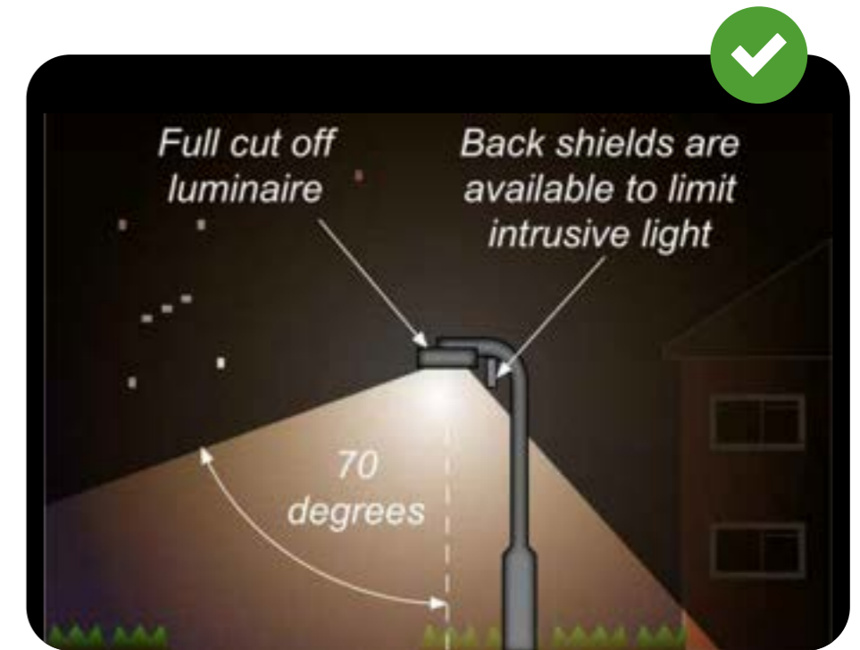
Typical well directed full cut-off street lighting, with shields (image courtesy of Commission for Dark Skies)
